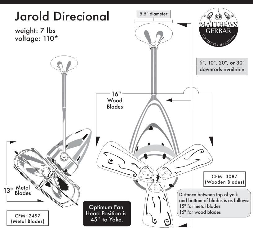
The Jarold Directional can be mounted with any one of the following downrod lengths: 5, 10, 20 or 30".
