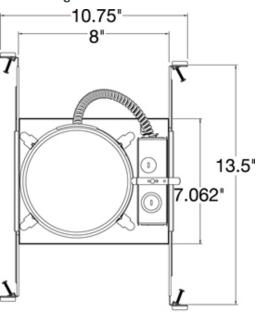
New Construction Shallow IC Airtight Housing
